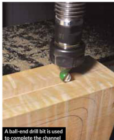
A ball-end drill bit is used to complete the channel
