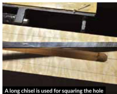
A long chisel is used for squaring the hole
