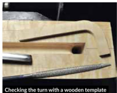
Checking the turn with a wooden template
