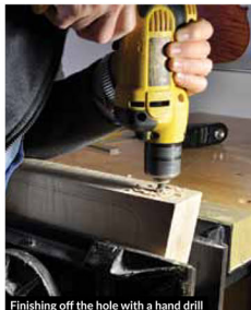
Finishing off the hole with a hand drill
