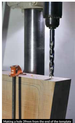
Making a hole 39mm from the end of the template
