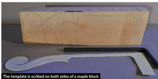
The template is scribed on both sides of a maple block
